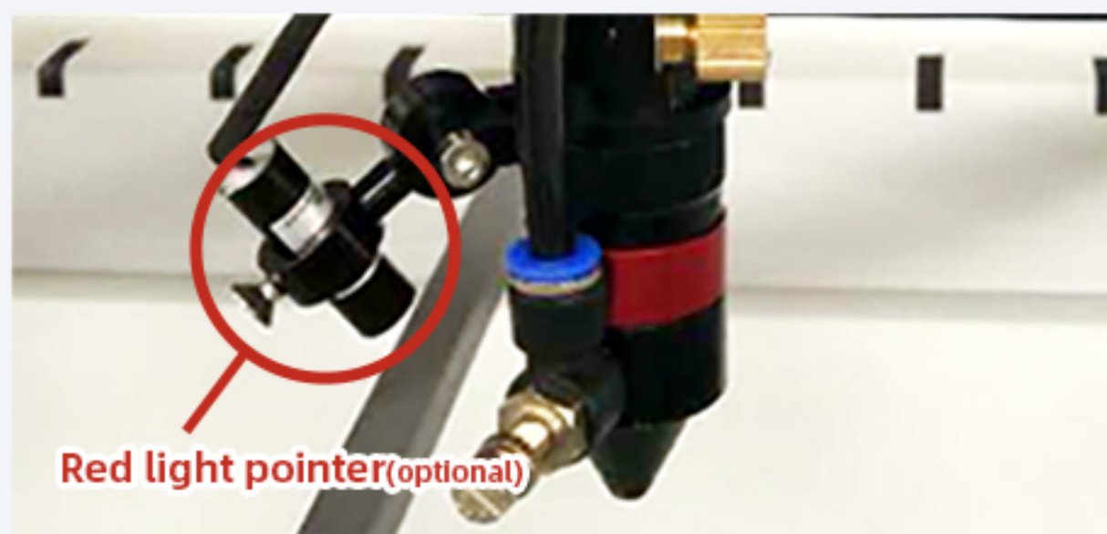
Laser is invisible, Red laser beam to determine the cut-off point
